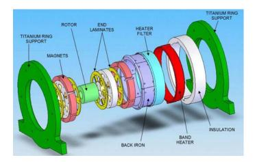
Figure 6 Stator Sub-Assembly
