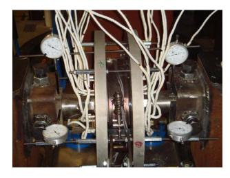
Figure 9 Alignment of the Force Test Fixture
