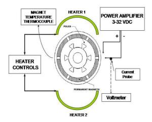
Figure 8 Schematic of the test setup
