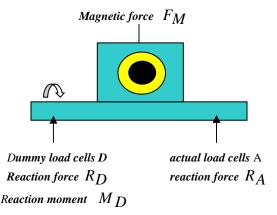
Figure 13 Schematic of 2 load cell setup
