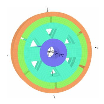
Figure 1 Solid Model of the Radial Bearing
