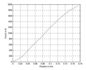
Figure 14 Measured Force vs. Position with Zero Current
