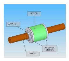
Figure 7 Rotor Sub-Assembly
