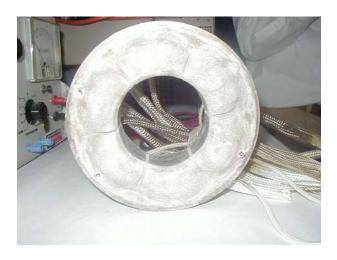
Figure 12 View of Inner Face of Stator with High Pot Instrument
