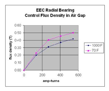
Figure 4 Flux density vs. Amp-turns
