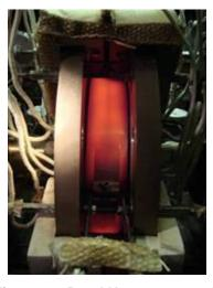
Figure 11 Band Heater at 1,000F
