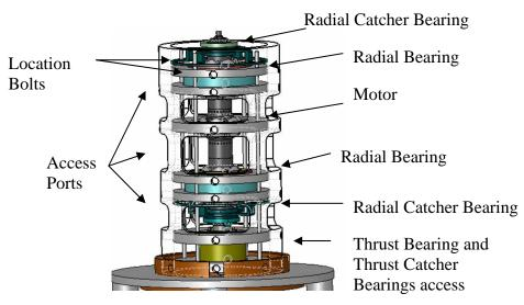
**Figure 17 High Temperature Test Rig Components**
