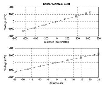
Figure 18 High Temperature Displacement Sensor Calibration
