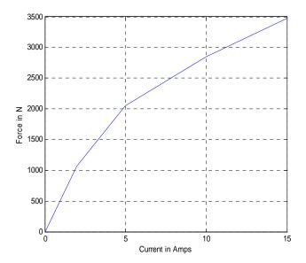
Figure 15 Measured Force vs. Current with Fixed Position
