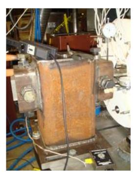
Figure 10 Monolithic shaft support
